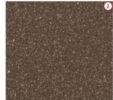
Fig 02: Proposed External Door, Window, Railing and Aluminium Cladding Finish - Syntha Pulvin Bronze or similar
